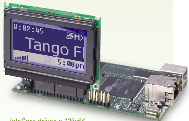
lalaCore drives a 128x64 graphics LCD module
